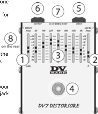
**ON/OFF SWITCH\* (4)** – turns the effect on and off; the LEDs on the sliders illuminate when the effect is on.
